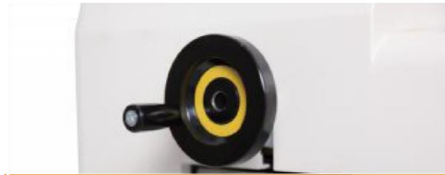
Set jaw plate gap by rotating handle
